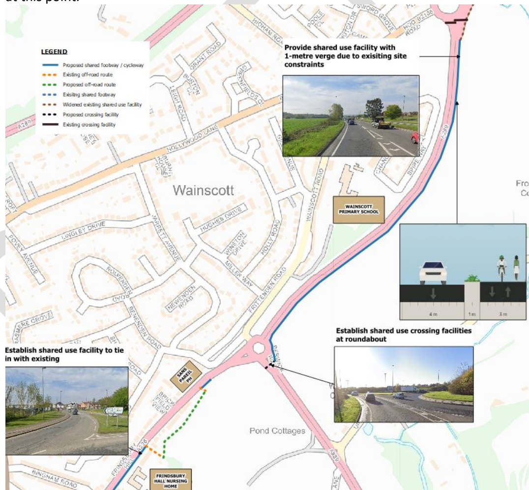
Figure 6 Interventions for Cycle Route 9 - Four Elms Hill to Sans Pareil roundabout, Chattenden
