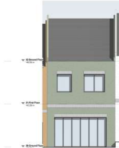
2 Townhouse - 2B3P - Rear Elevation Scale: 1:50
