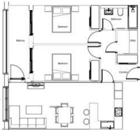
APARTMENT TYPE 4 (TYPE 100) Total GFA 31.5sqm Entrance Hall 3sqm Lounge 20sqm Bedroom 1 12sqm Bedroom 2 10sqm Bathroom 4sqm Library 3sqm Balcony 2sqm
