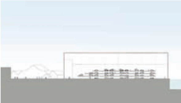
Section illustrating tiered car park structure
