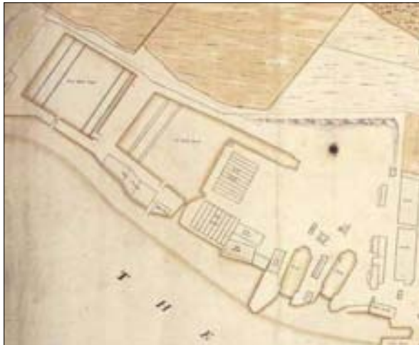
Plan showing the layout of the dockyard in the early 18th century with the two mast ponds and the sea wall clearly visible.
