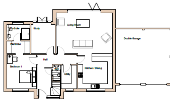
Ground Floor Plan - Plots 1 & 2 100.39 sq m (1080 sq ft) Total Floor Area = 177.62 sq m = 1912 sq ft
