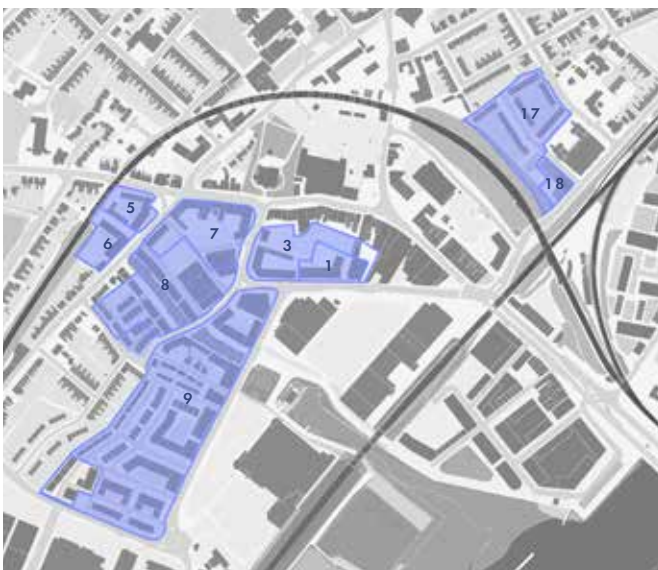
The density proposed by the illustrative masterplan is approximately 100 dwellings per hectare across the residential sites (shown above).
