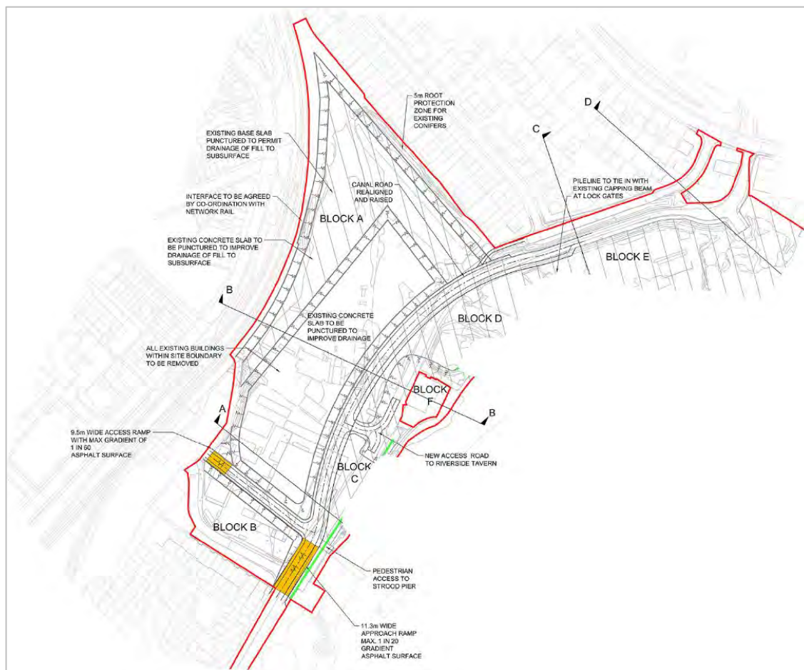
Figure 5-9: Clip of general arrangement of rear boundary and central portion of the Phase 2 site
