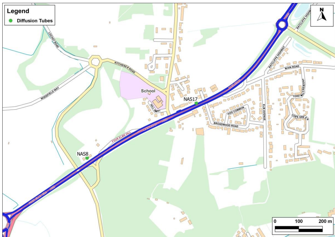
Figure 1 Detailed Assessment Study Area and Monitoring Locations. Roads explicitly included in the model shown in blue.
