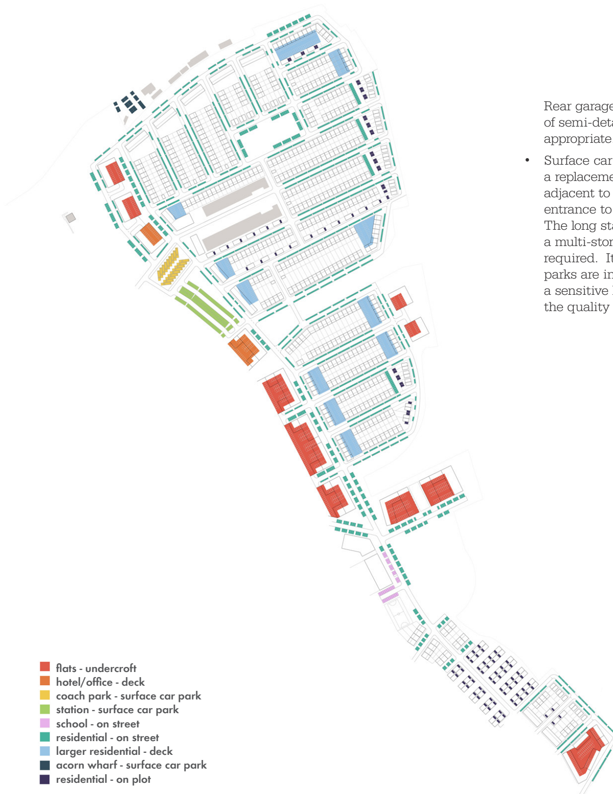
Parking types - indicative parking arrangements based on the illustrative mix of housing typologies and uses in the current masterplan
