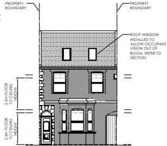
PROPOSED FRONT ELEVATION (SCALE 1:100)
