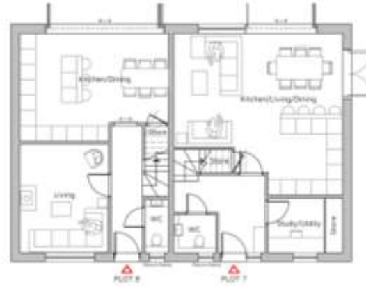
Proposed Ground Floor Plan 1:100 @ A3
