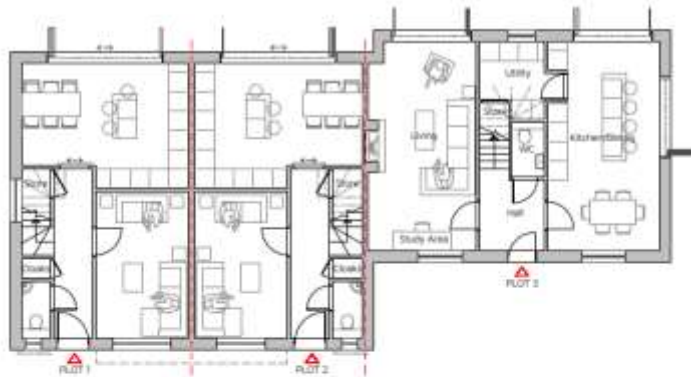
Proposed Ground Floor Plan 1:100 @ A2
