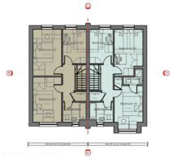
First Floor Plan As Proposed HTD - 385P - GFA = 48.34m 2 (per plot) / HTE - 385P - GFA = 50.75m 2 (per plot) 1100
