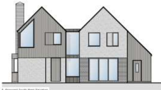
1. Proposed South West Elevation 1:100 @ A3
