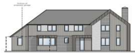
1. Proposed North West Elevation 1:100 @ A3
