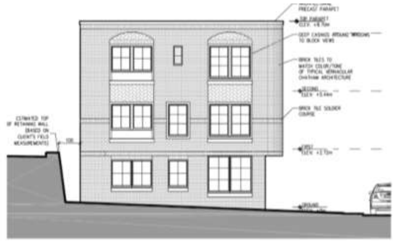
1 EAST ELEVATION (THE MOUNT) 1:100
