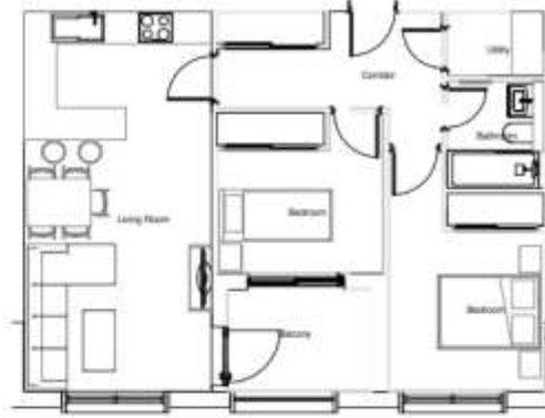
APARTMENT TYPE 2 (2 BED ROOMS) Total GFA 61.2sqm Entrance Hall 8sqm Lounge 12sqm Bedroom 1 12sqm Bedroom 2 12sqm Bathroom 4sqm Library 3sqm Balcony 1sqm
