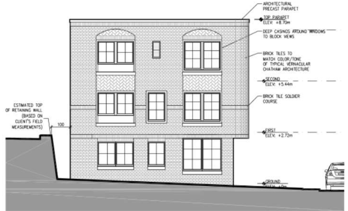
1 EAST ELEVATION (THE MOUNT) 1:100
